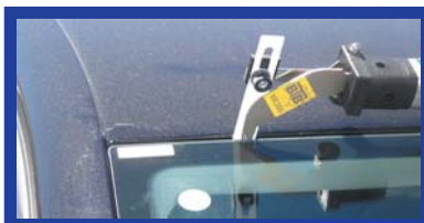
WK11PP arm with external cutting WK28 blade
