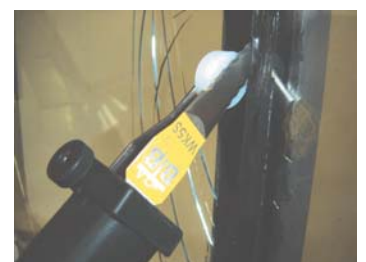
Removing backfill urethane between bus window glasses
